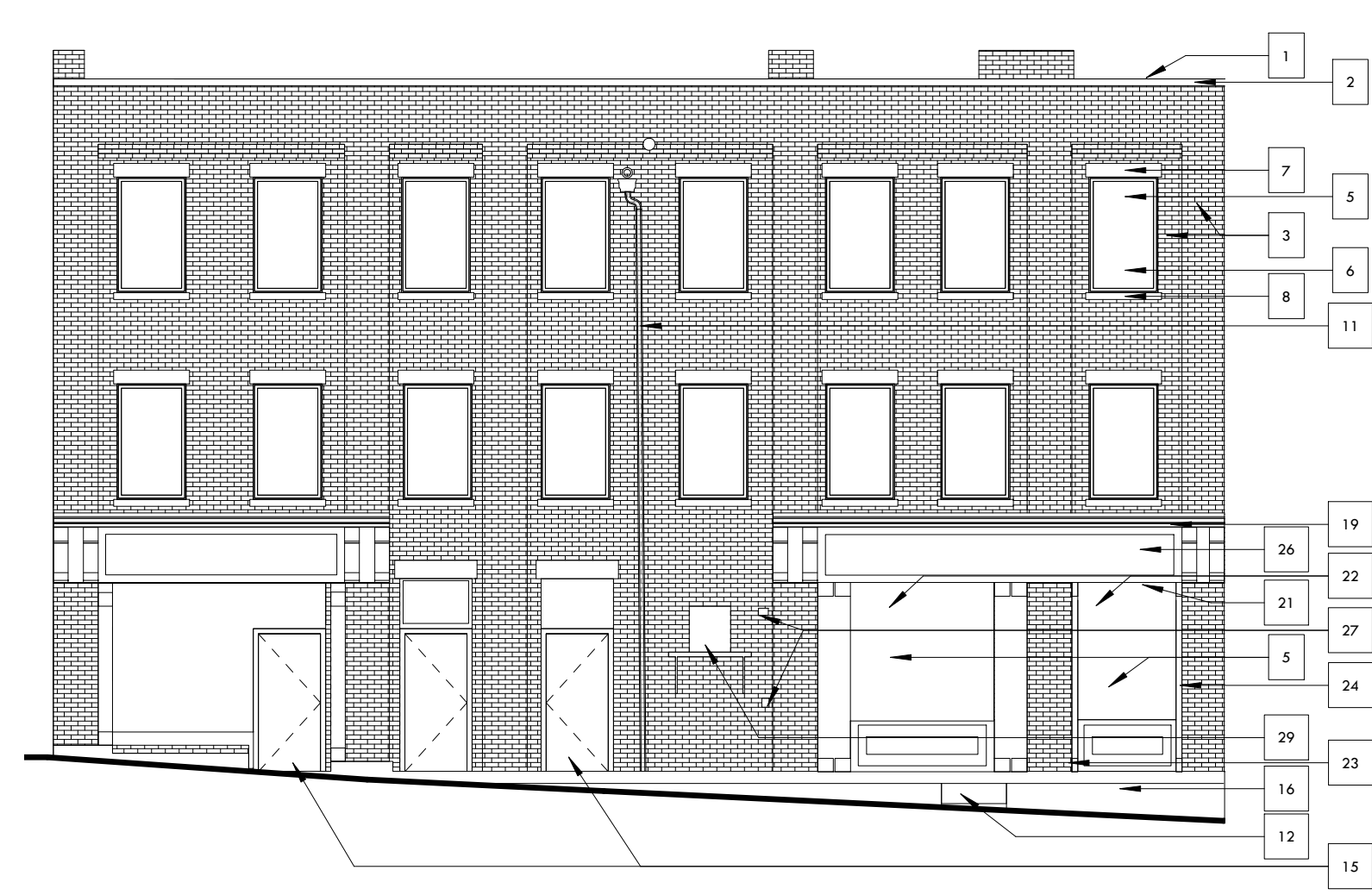
3 EXISTING EAST ELEVATION - KIRKPATRICK STREET 1/8" = 1'-0"
