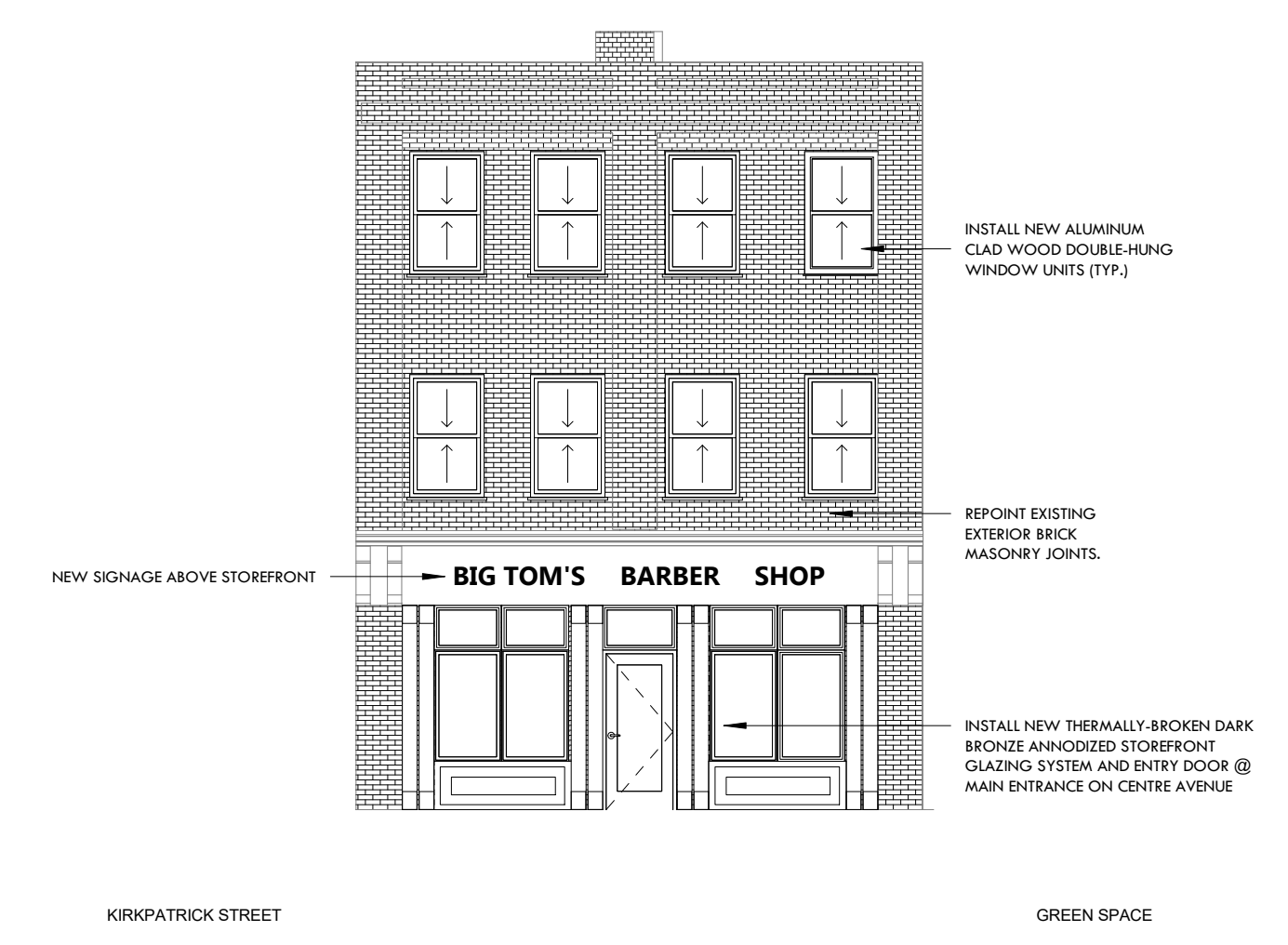
1 PROPOSED NORTH ELEVATION - CENTRE AVENUE 1/8" = 1'-0"
