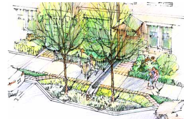
FIGURE 2.7 Precedent sketch showing roof runoff channeled to bioswales in curb bumpout planters
