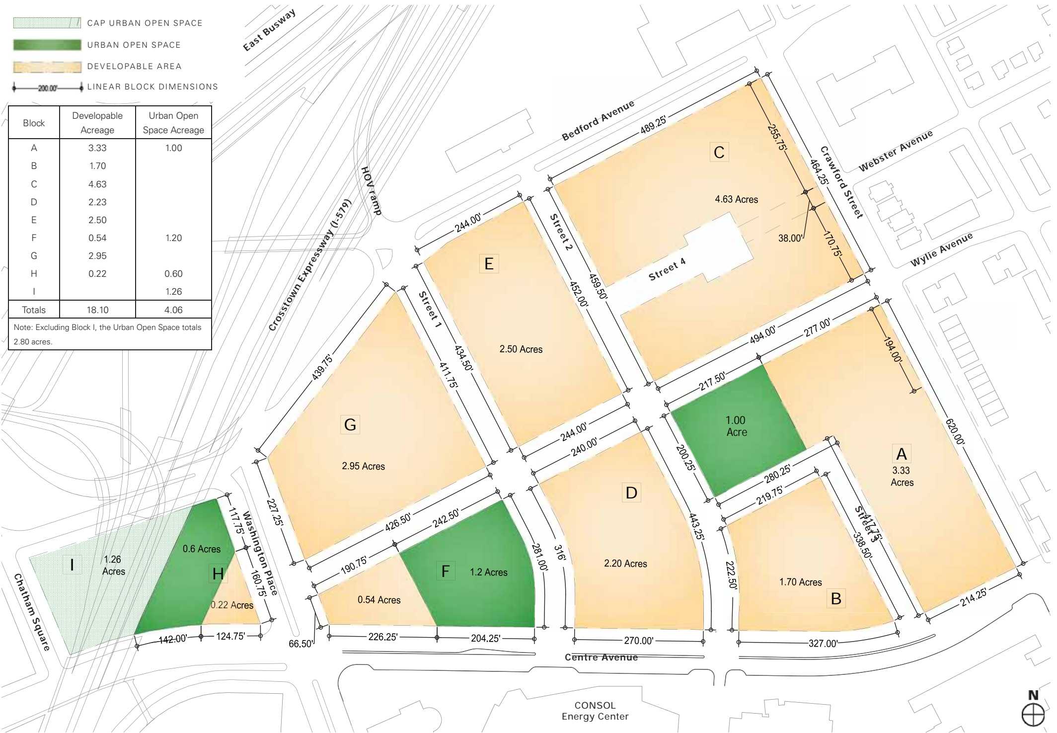
FIGURE 2.11 Block Regulating Plan Note: All dimensions and area quantifications are based on available GIS data and are horizontal measurements. Consult final site survey for accurate data.
