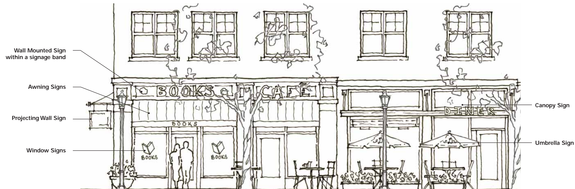
FIGURE 6.8 Elevation illustrating the various building signs that may occur along a facade
