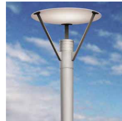
FIGURE 6.23 Example of street/ pedestrian-scale LED post light that incorporates indirect light to comply with Dark Sky Regulations.
