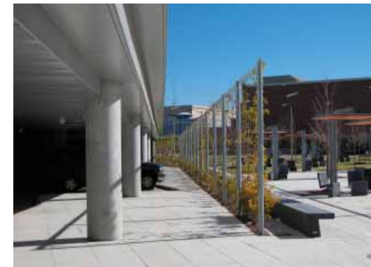
FIGURE 2.39 When facing the interior of a block, podium or garage parking may be screened by landscape in place of an architectural facade. In this example, a layering of sidewalk, landscape and benches create an effective and attractive screen.
