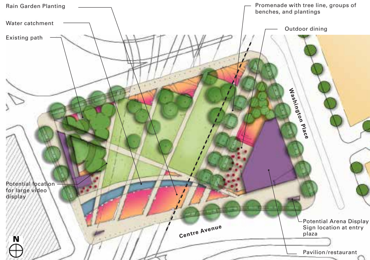
FIGURE 7.3 Enlarged illustrative plan showing a small adjacent pavilion/restaurant with an outdoor dining terrace, pylon marking the entry plaza, and a tree-lined promenade.
