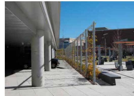
FIGURE 2.67 When facing the interior of a block, podium or garage parking may be screened by landscape in place of an architectural facade. In this example, a layering of sidewalk, landscape and benches create an effective and attractive screen
