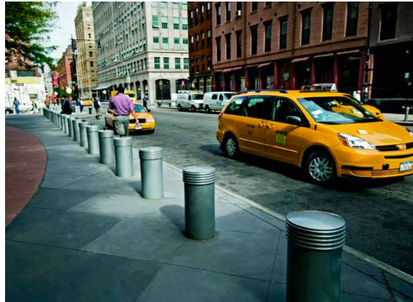
FIGURE 6.17 Example of security bollards (Landscape Forms).
