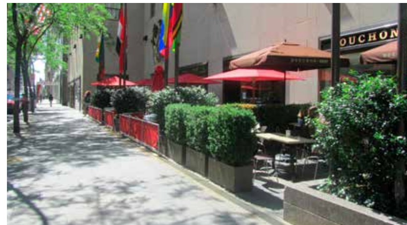
FIGURE 6.14 Example of cafe barriers using fence panels and moveable planters adjacent to the sidewalk. Note the permanent planter that holds the corner of the ROW line and reflecting the architecture of the building.
