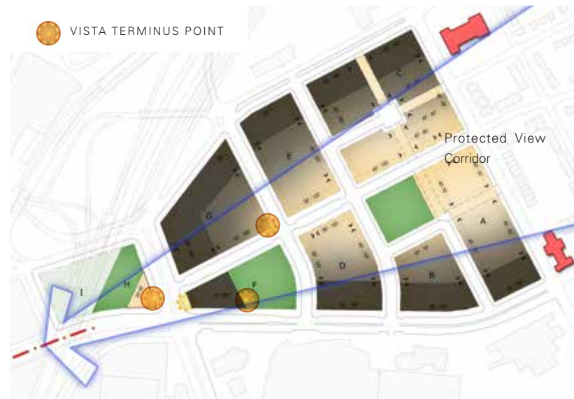
FIGURE 2.55 Diagram of desired view corridor through the site. This view corridor is codified by the height limits described on the page that follows.
