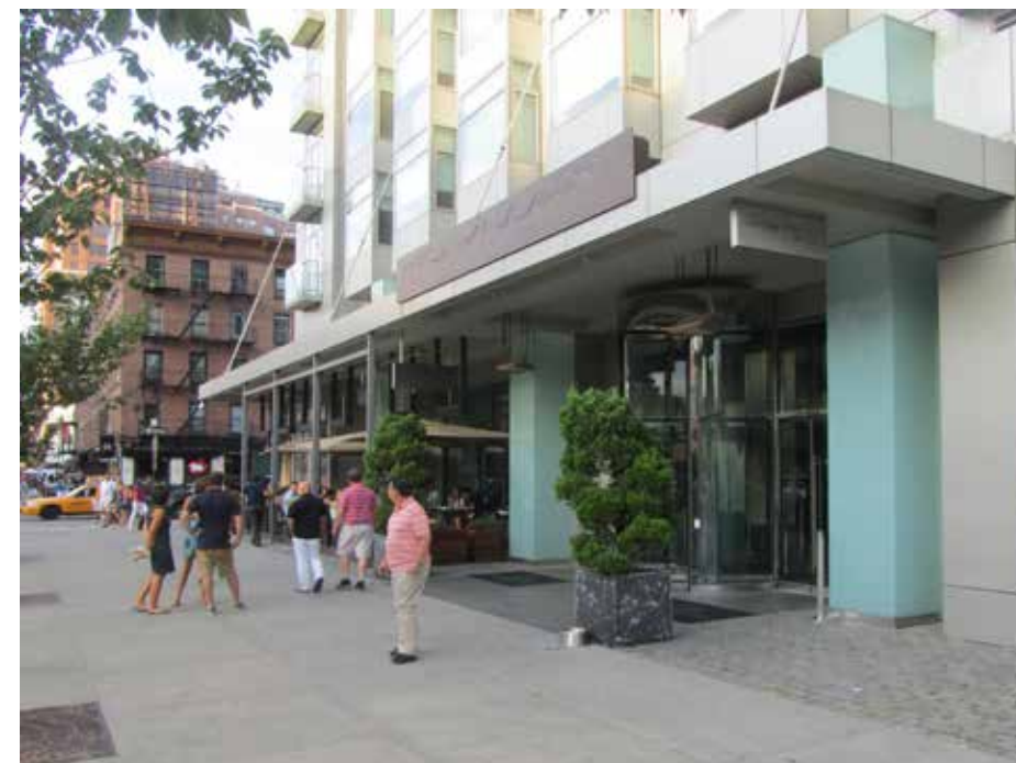
FIGURE 2.48 Typical commercial/residential frontage showing recessed entry and covered outdoor seating. Overhang extends to setback line and helps building maintain the sidewalk edge.
