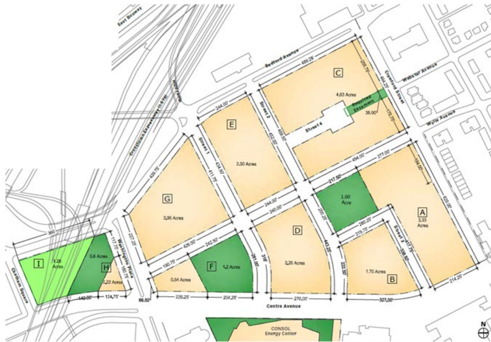
FIGURE 2.24 Block Regulating Plan Note: All dimensions and area quantifications are based on available GIS data and are horizontal measurements. Consult final site survey for accurate data.
